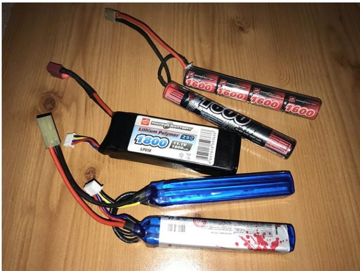
NiMH (nickel-metal hydride) are the 'standard' batteries which require a basic charger and are very safe to use. The disadvantage is that the large NiMH batteries are bulky and require a large space inside the AEG to store them (such as inside a solid stock). Small NiMH batteries overcome the size issue but do not last for long so you will find the battery will run out after 1000 rounds or so and you have to swap it mid game. AEG's are usually designed to run on 8.4 volt NiMH batteries.
